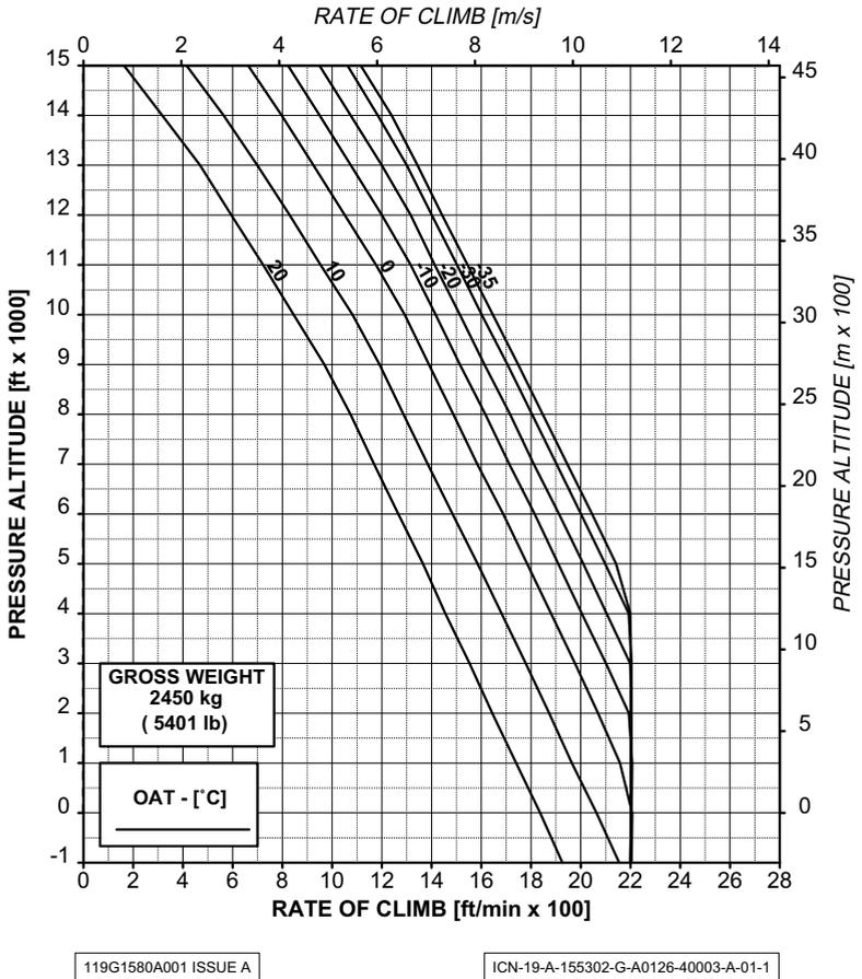
**Figure 4-7. Take-Off Power (TOP) (Heater On)
