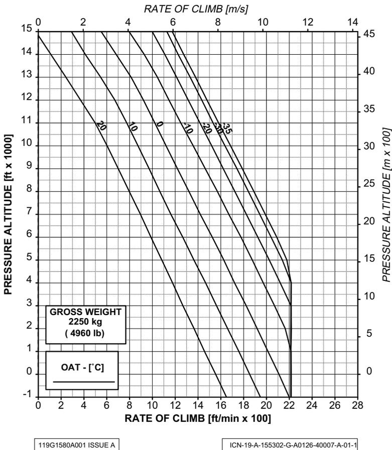
**Figure 4-11. Maximum Continuous Power (MCP) (Heater On)**
