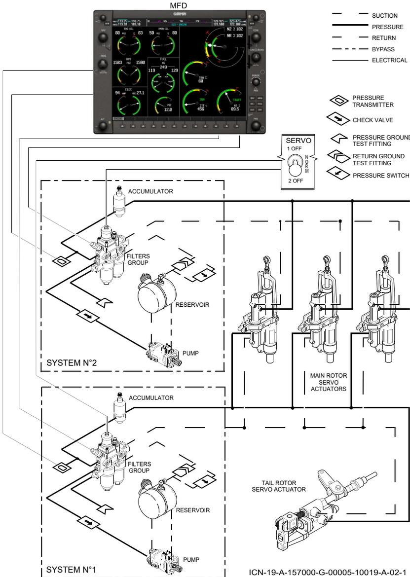
Figure 7-21. Hydraulic Power Schematic
