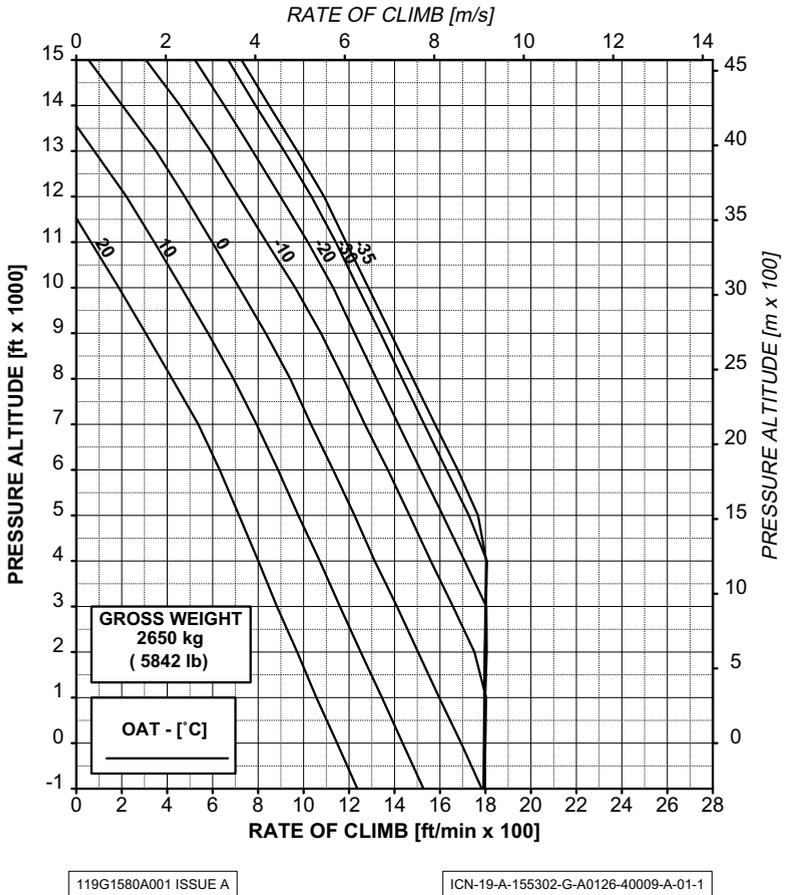
**Figure 4-13. Maximum Continuous Power (MCP) (Heater On)
