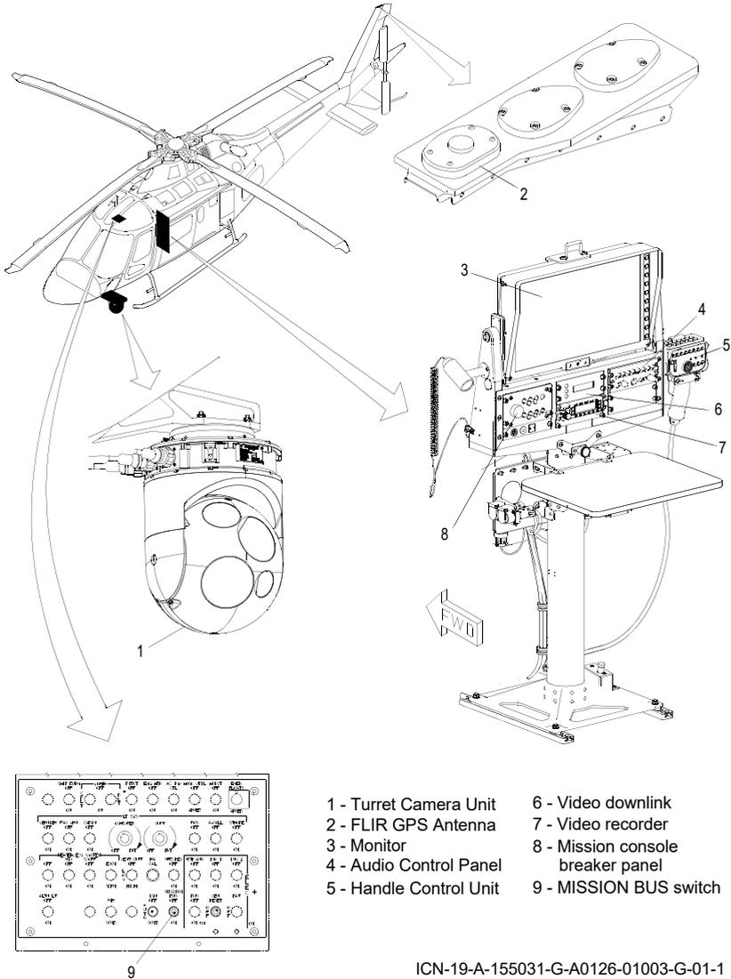
**Figure 7-1. Flir MX-10 installation (G1000H NXi only)
