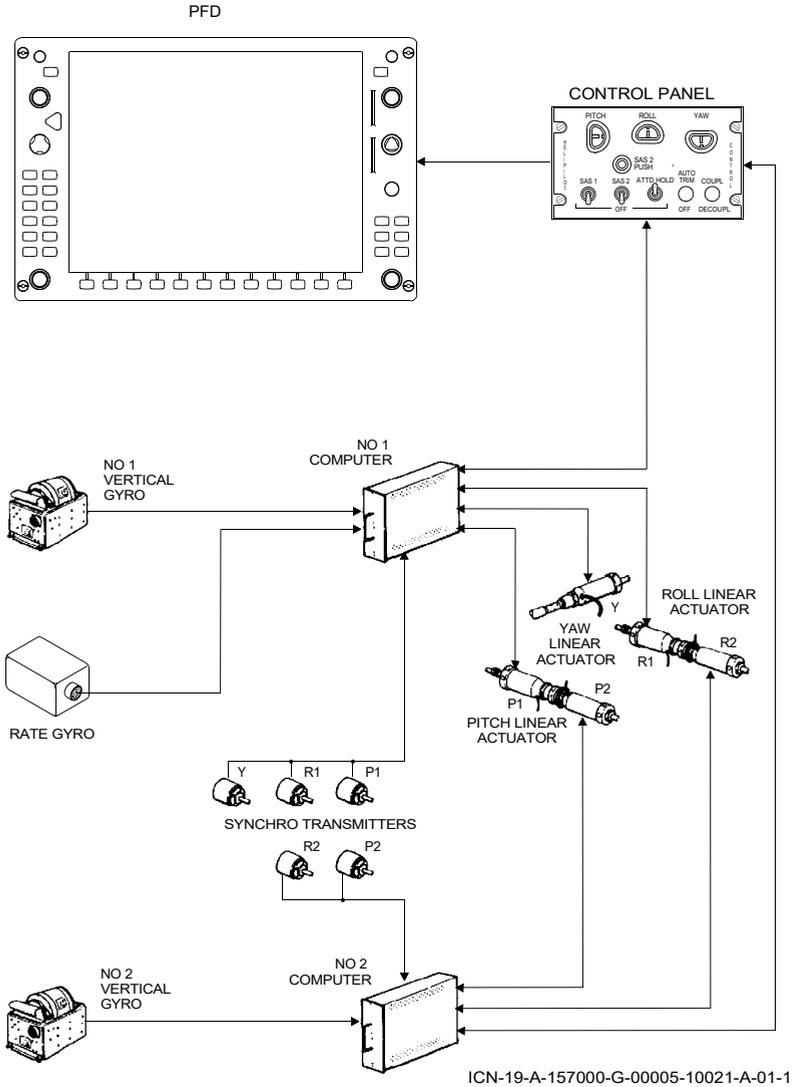
Figure 7-23. Helipilot System Schematic
