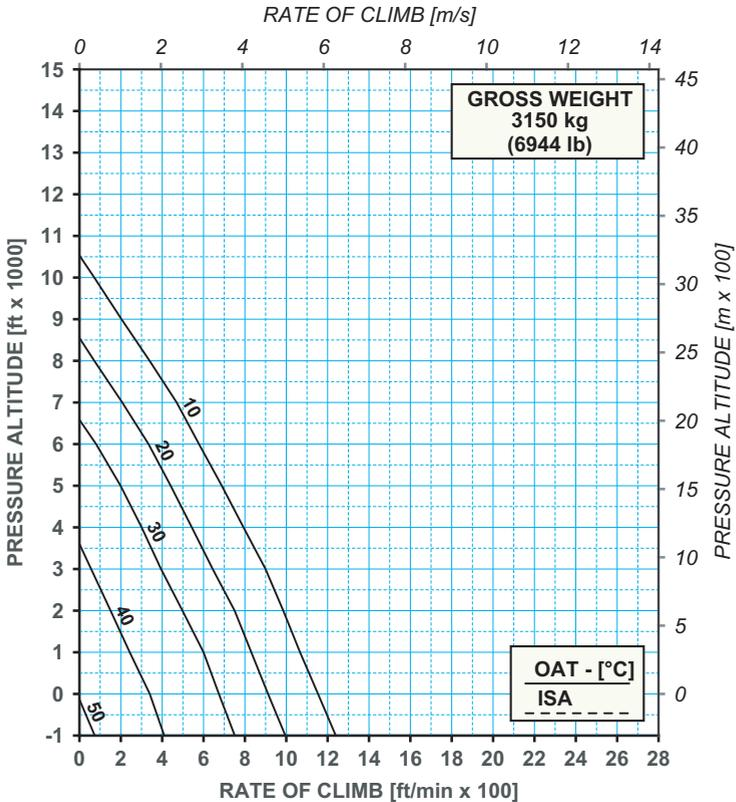
**Figure 9-98. Rate Of Climb - Maximum Continuous Power (MCP)**
