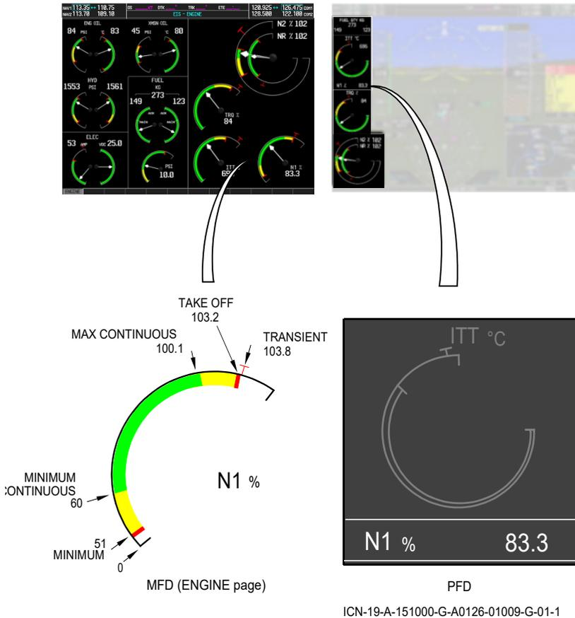
Figure 1-12. Gas Generator Speed (N1)
