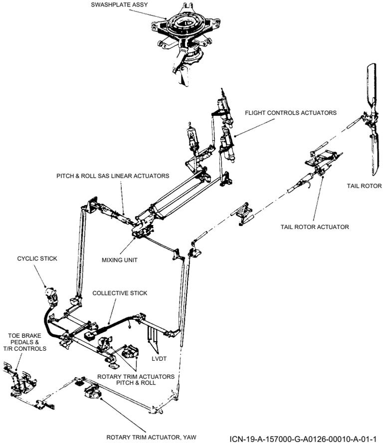
Figure 7-18. Flight Controls System
